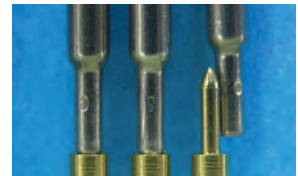
The X Probe may have missed the termination pin and is not making the connection. Remove the X Probe, verify plate alignment and re-install.
