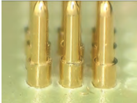
Sheared off retention beads leave metal shavings that could cause electrical shorts.
