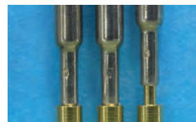
If the X Probe is sitting too high, it may not be seated properly. Continue pushing down until the connection is complete.
