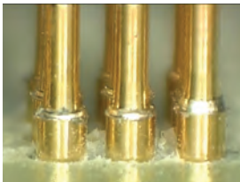
Damage to the shoulder of the termination pin and inconsistent set heights can occur with undersized holes or excessive hammering.
