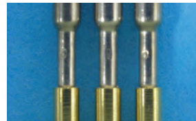
Proper X Probe installation, bottom of probe tube is sitting on shoulder of Termination pin.
