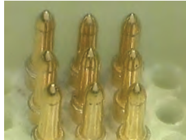
Mounting plate material may be displaced due to excessive hammering.
