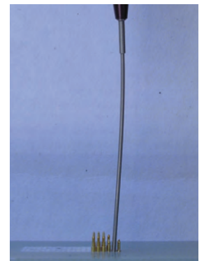
Incorrect use of tool. ETRX-E tool may buckle.
