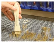
QA uses a small amount of lubricant to minimize wear caused by the internal sliding contact surfaces of our probes. Never use cleaning solvents on your probes as it may wash particles down into the critical internal surfaces. This could affect the performance and shorten the life of your probes.
