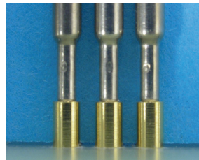
Proper X Probe installation, bottom of probe tube is sitting on shoulder of Termination pin.
