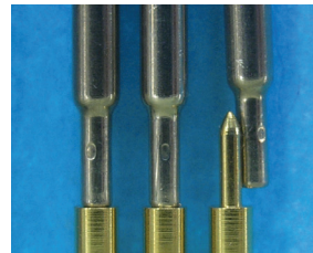
The X Probe may have missed the termination pin and is not making the connection. Remove the X Probe and re-install.
